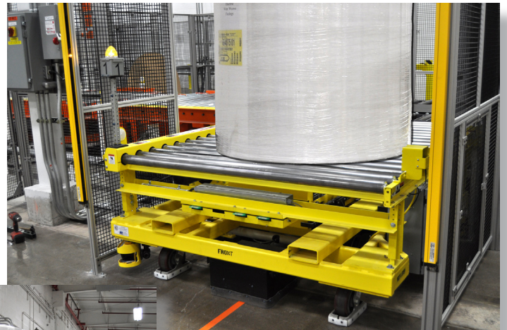
A Titan Designed Automated Guide Vehicle for a major consumer product manufacturer carrying rolls of plastic from workstation to warehouse.
