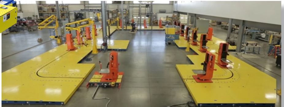
Floor Guided system for assembly of marine engines
