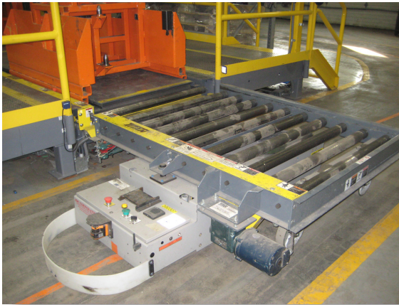
A Titan Designed Automated Guide Vehicle for a major defense contractor carrying diesel engine components from workstation to workstation.
