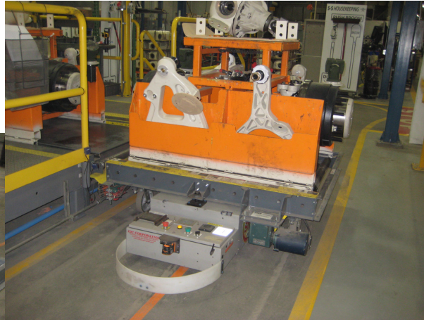
A Titan Designed Automated Guide Vehicle for a major defense contractor carrying diesel engine components from workstation to workstation.
