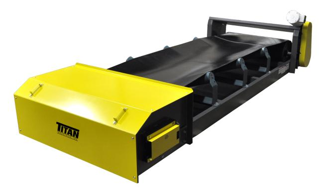
The Model 460 Bulk Handling Conveyor is specifically designed to handle large volumes of heavy, abrasive and granular products at a very reasonable cost. The Model 460's rugged construction and certified components provide for long runs and outdoor applications. Carrying 3 roll idlers are spaced on 4' centers in the intermediate section and spaced closer at each terminal. Infeed hoppers, skirting, belt scraper and supports are some of the available options.
