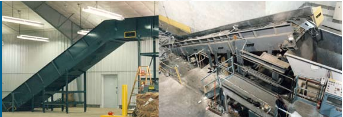
5. Stitch Weld H.D. angle iron gussets on all extended side rails for conveyor strength and esthetics.
