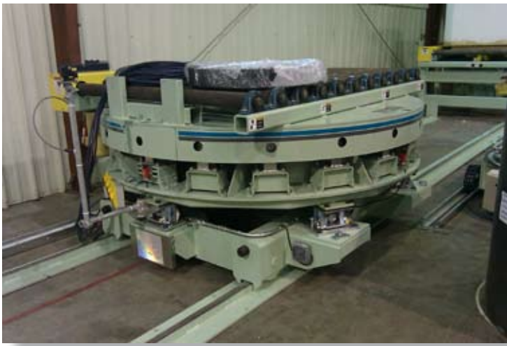
Extreme duty turntable on rail guided cart
