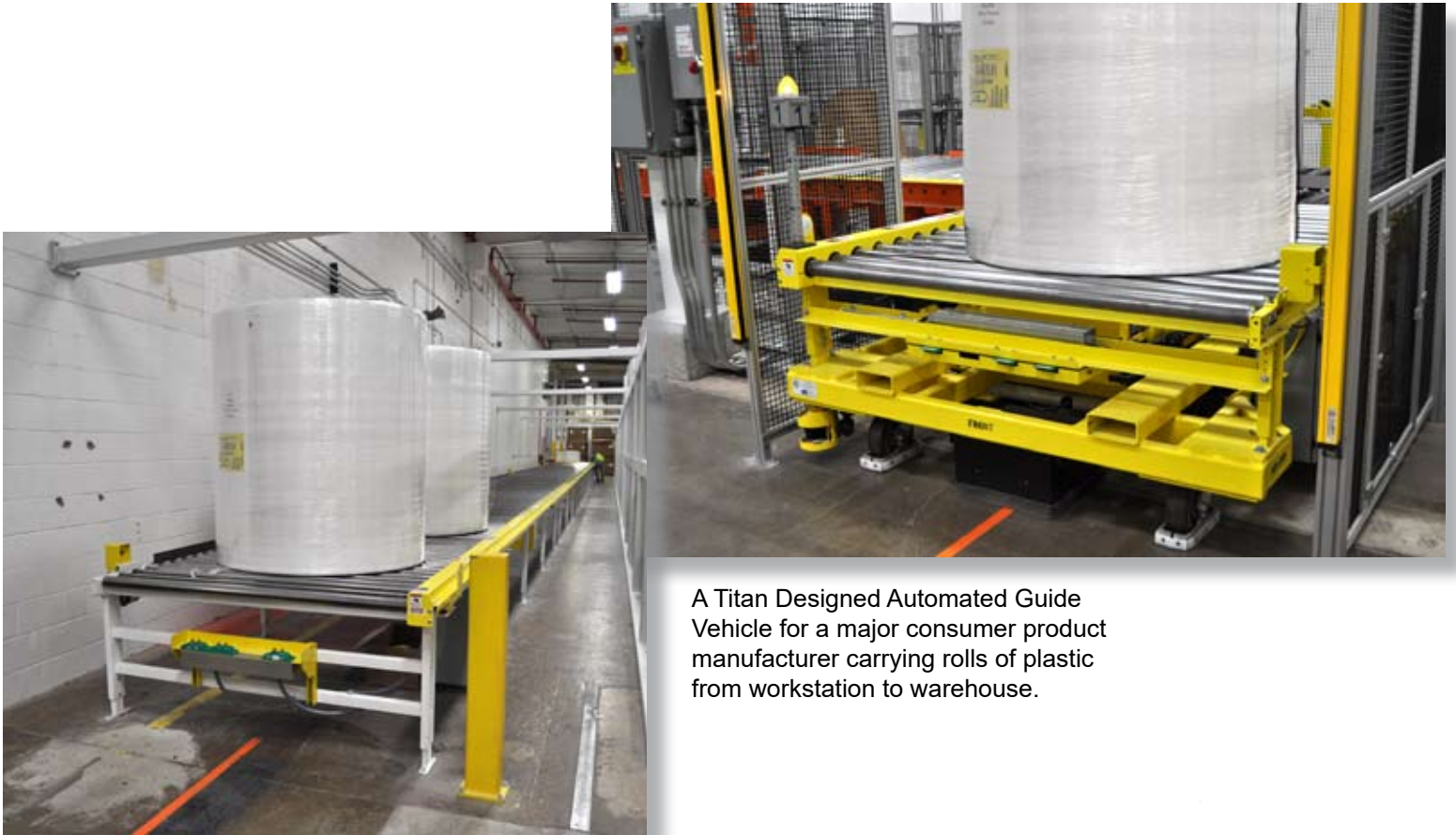
Extreme duty turntable on rail guided cart
