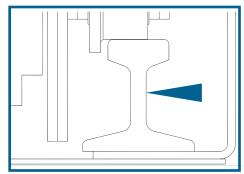
1. H.D. 25# rail track reduces wear factors and improves conveyor integrity.
