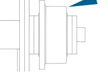
2. 3" diameter bushed single flanged rollers. Sintered metal composition allows for closer machining tolerance and improves wear factors.
